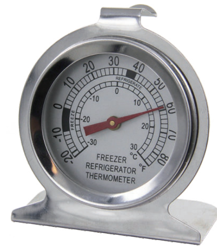
Model:ZLB-467B Bimetal Fridge Thermometer SIZE:70*62*40mm Material:Stainless Steel
